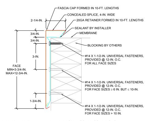
PRE-DRILL WITH 3/16-IN. DRILL BIT FOR MASONRY CONDITIONS. CONTACT OMG FOR APPROPRIATE RECOMMENDATIONS NEEDED TO MEET/EXCEED ANSI/SPRI/FM4435/ES-1 DESIGN CRITERIA
